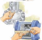
• Document the shaft or stem diameter, stuffing box bore and depth, and, when using lantern rings, distance of port to bottom of stuffing box.
